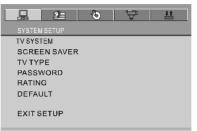
2 Press the LEFT or RIGHT button to highlight the icon of the desired page, then press the DOWN or UP button to activate that page.
